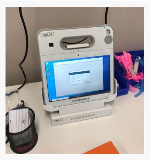
It came with the option to include a 2D barcode scanner, RFID reader and fingerprint reader built right into the device. The full-sized ports also made it easy to integrate the Emirates ID card reader.
